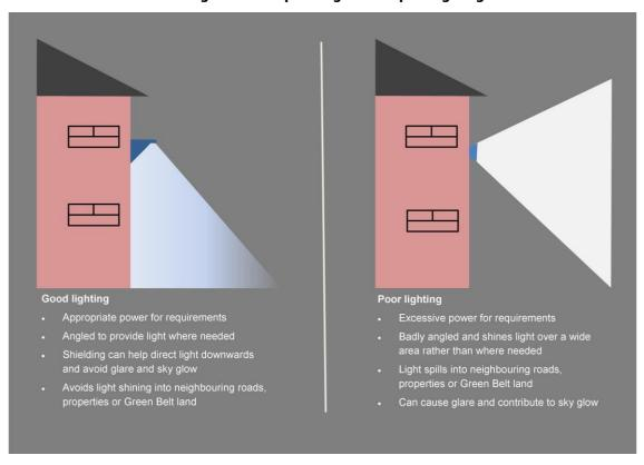
Figure 4 Examples of good and poor lighting
